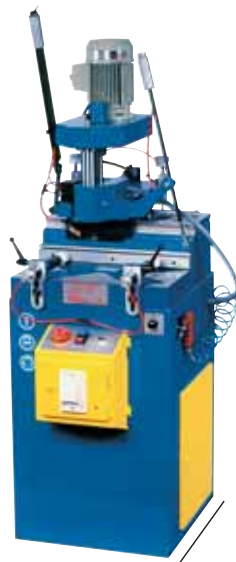
C 500 A Desp. vertical 100 mm Desp. longit. 260 mm - Desp. trans. 100 mm
